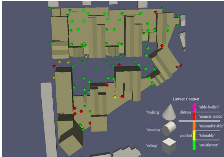
Figure E2: Lawson comfort criteria within the proposed development excluding any landscape features or other mitigation measures
