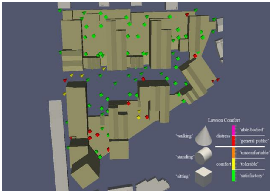
Figure 5.2: Lawson comfort criteria within the proposed development excluding any landscape features or other mitigation measures
